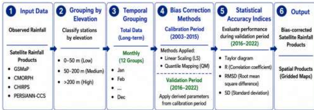
Figure 2. Overall methodological framework for satellite rainfall bias correction and performance evaluation under long-term and monthly parameterization approaches.
